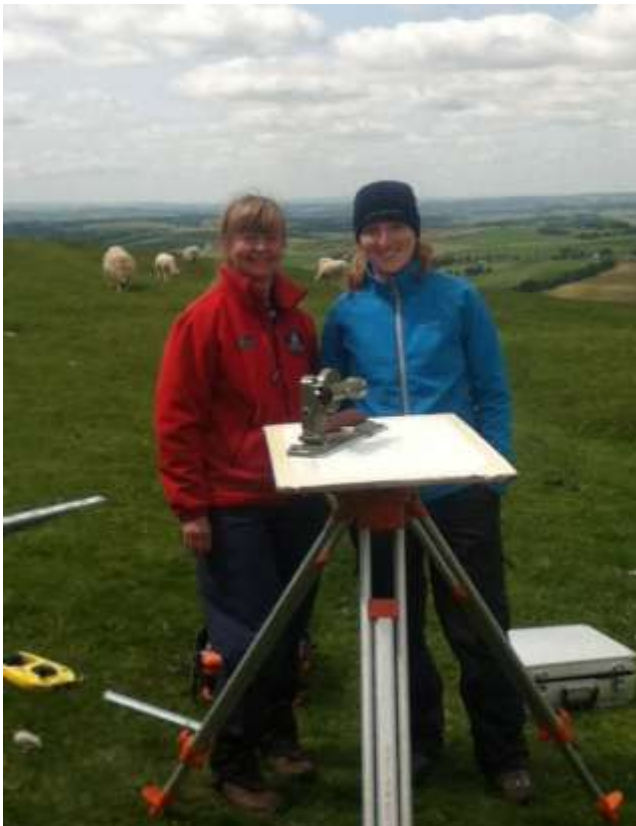
Fig 1: Plane table survey of the SSE terminal of the newly discovered cursus
